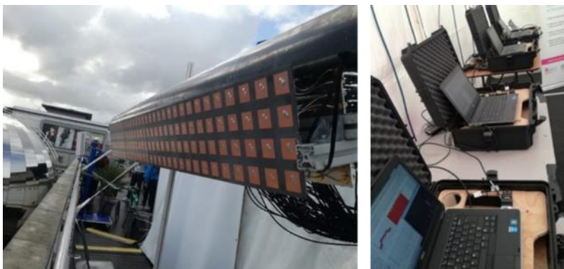
Figure 70: Massive MIMO test network at the Smart Internet Lab
